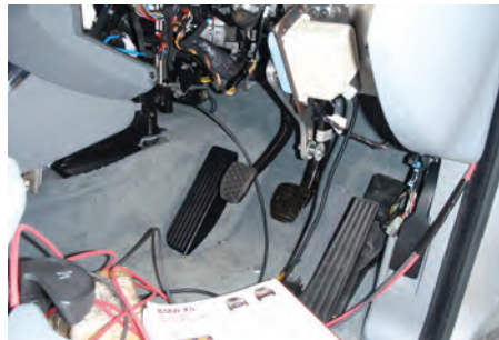
Above: The brake-pedal electric servo in the BMW
